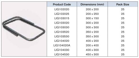
Standard size ligatures for tying reinforcing bar or trench mesh. Manufactured from plain round bar Grade R250N to AS/NZS 4671.
