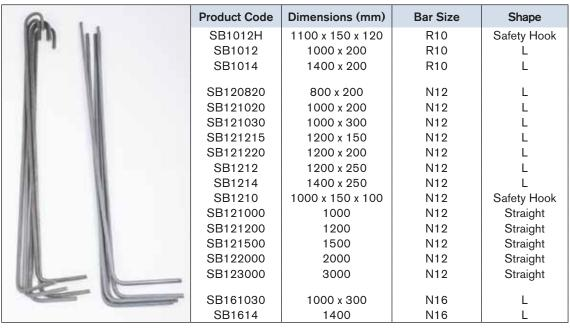
Standard cut and bent deformed bar Grade D500N to AS/NZS 4671.
