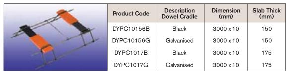
Danley® Plate Dowel Cradles consist of a plate dowel secured in a fabricated cradle, offering a highly efficient dowel system well suited for contraction joints. Dowels available in black, galvanised and stainless steel (on request).
